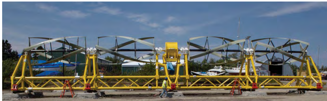
Figure H-19. ORPC TidGen Tidal Generator
