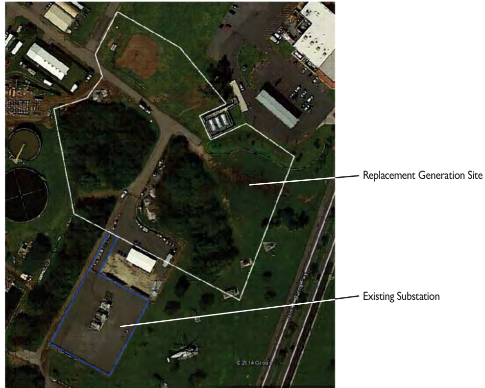
Figure D-1. MCBH Site for Possible Replacement Generation
