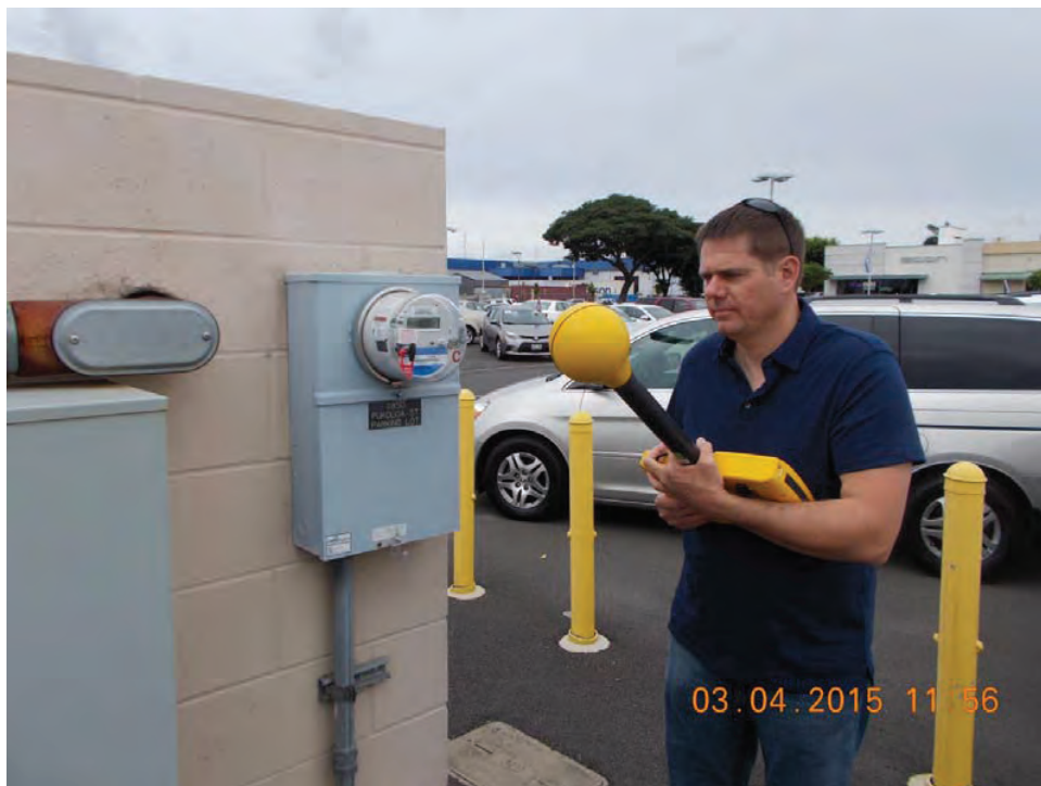
Figure 2. Measurement of smart meter fields at site 10.
