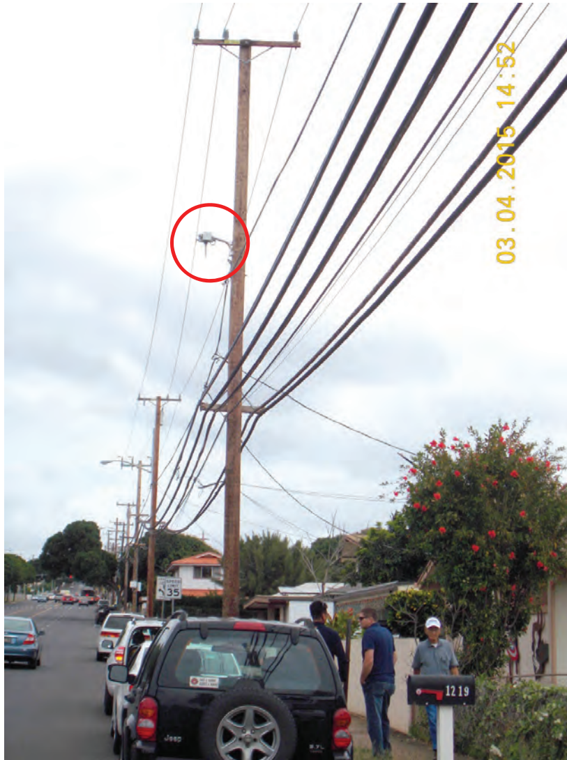
Figure 5. Location of an access point (AP) installed on an electric power pole at site 12 (see red circle). Measurements were performed along the edge of the street in one direction from the power pole.
