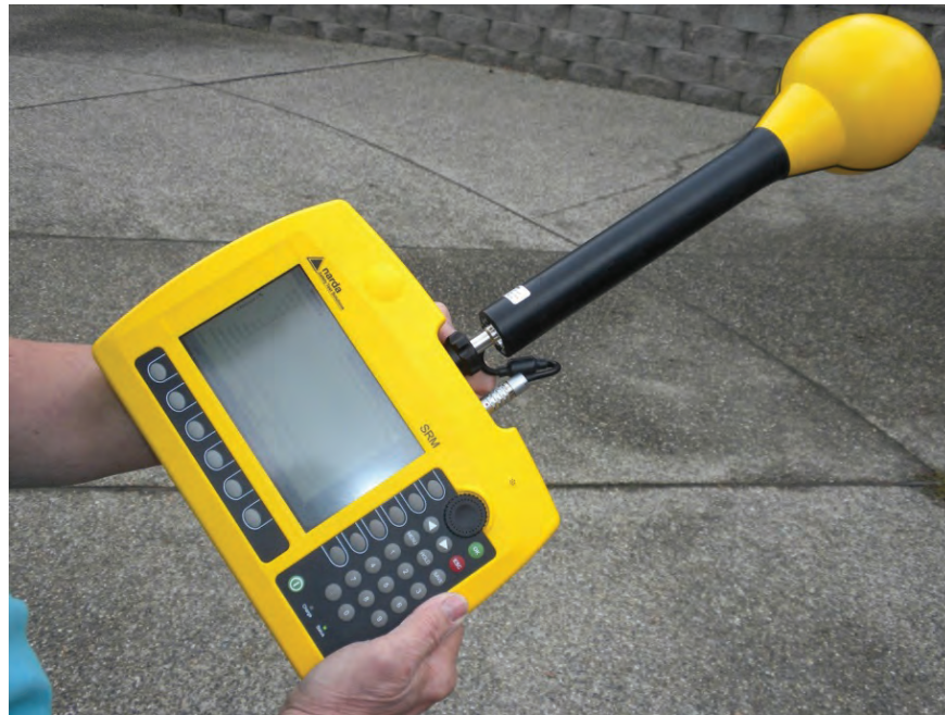
Figure 6. The Narda SRM-3006 Selective Radiation Meter is based on Fast Fourier Transform (FFT) spectrum analyzer technology and uses a probe/antenna to measure the absolute magnitude of incident RF fields across the frequency range of 26 MHz to 3,000 MHz and digitally converts the detected field to the equivalent percentage of the FCC MPE.
