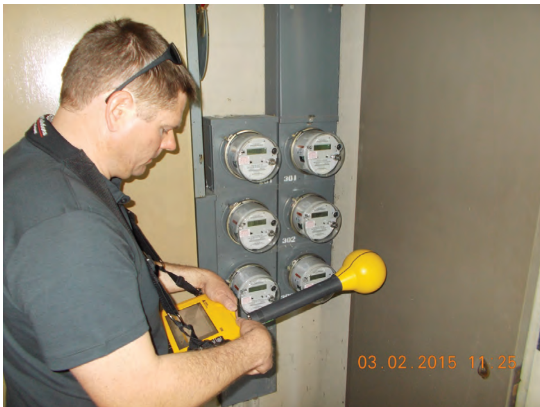
Figure 3. Illustration of the measurement of RF fields at a bank of six meters at site 7.
